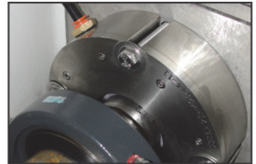
The AM Food Grade is a permanent shaft seal made of food grade materials for applications in the food processing industry.
