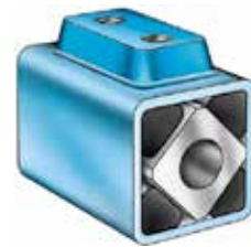
Fig. 6 Dual-threaded plate welded on housing
